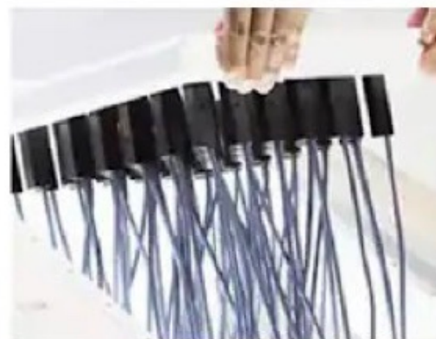
Bio-magnetic sensors arranged in an array for measuring the cardiac magnetic field
